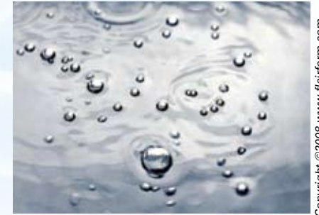
High \text{CO}_2 levels are evident from the formation of bubbles in a bore water sample. The pH will rise as the \text{CO}_2 escapes
